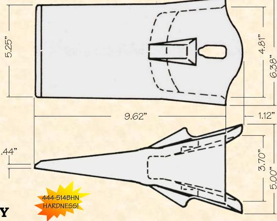
Uses the C-50 Conical Series Rubber Insert and Steel Pin
