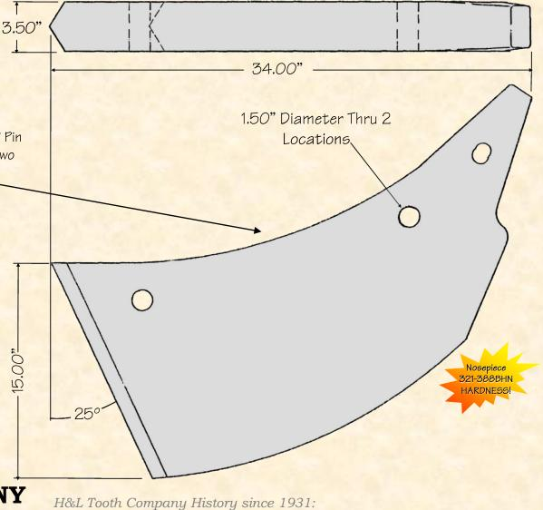
This H&L's RX-2114-AKYS-38 repair nosepiece was an offering by H&L style ripper conversion or repairs during the late 1970s. This Nosepiece uses H&L's 38 Series tooth system and was engineered, introduced by the H&L Tooth Company in 1972.
