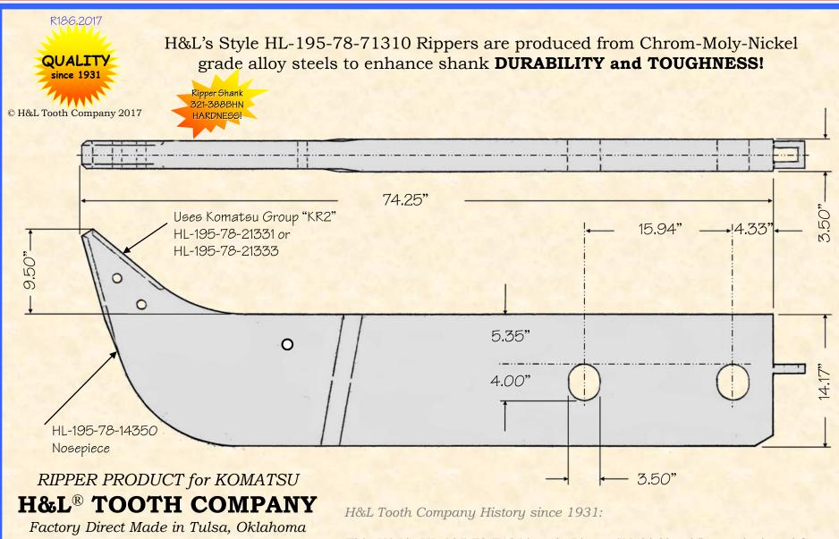
This H&L's HL-195-78-71310 style Ripper "Multi Shank" was designed for replacements of Komatsu machines dating back to 2004. Ripper Shank is used on Komatsu dozer, Models D375A-2 and D375A-5 with a box size of 3.75" X 14.50".
