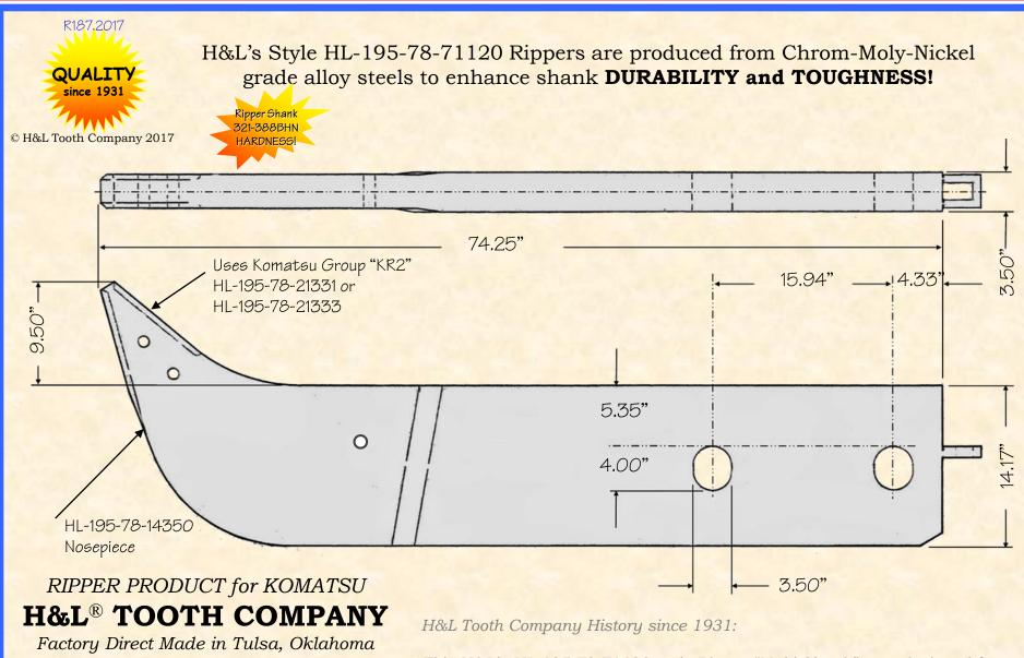
This H&L's HL-195-78-71120 style Ripper "Multi Shank" was designed for replacements of Komatsu machines dating back to 2004. Ripper Shank is used on Komatsu dozer, Models D375A-1 and D375A-5 with a box size of 3.75" X 14.50".
