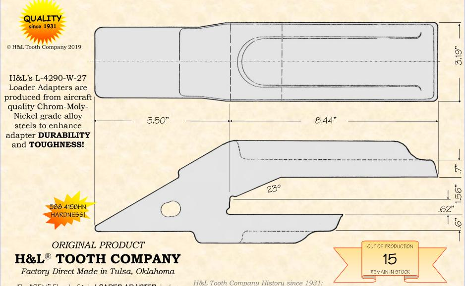
The "OEM" Flexpin Style LOADER ADAPTER design
