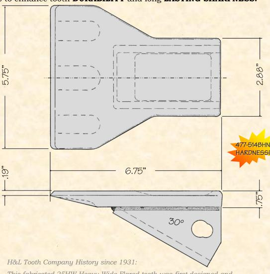
This fabricated 25HW Heavy Wide Flared tooth was first designed and introduced around 1934. This Flexpin type Tooth was first developed for an upgrade for a Page 3/4 Dragline and P&H model 150 Shovel, all before becoming the preferred standard on many models during the late 1930s.
