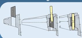
Installation of the Insert into the mining adapter, placement of the tooth, then hammer the steel pin through the tooth and nose, locking the pin to the Insert.
