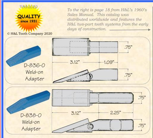
H&L's small trenching Adapters are produced from aircraft quality Chrom-Moly-Nickel grade alloy steels to enhance adapter **DURABILITY** and **TOUGHNESS!**
