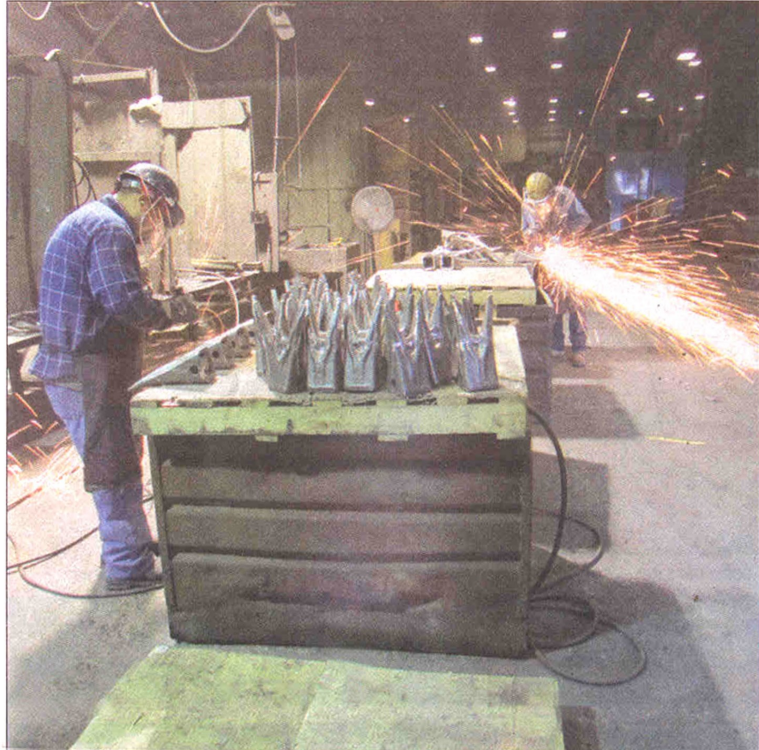
Finish forged part grinding.
