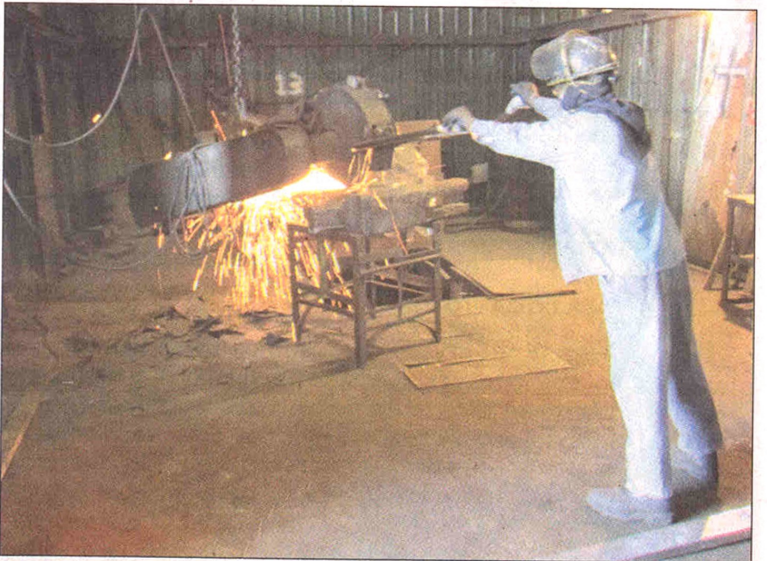
Swing ripper grinding.
