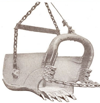
H&L Adapter type teeth in Esco Dragline bucket
