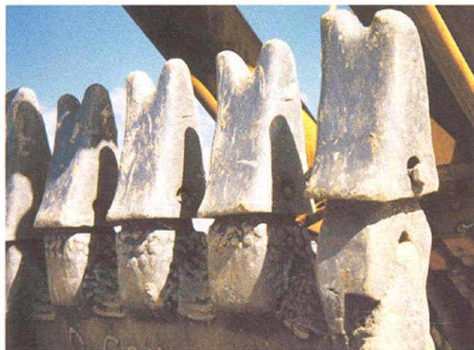
Top: Tooth blunting creates drag when trying to penetrate the digging bank. This requires greater machine power and accelerates hydraulic system and attachment bushing wear. Center: Note the attachment of the corner tooth instead of the pin and retainer as designed. Left: Poor welding can cause early failures and replacement.
