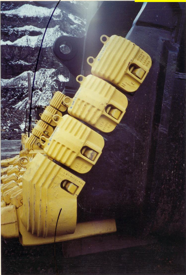
LX-4112-WSL Wing Shroud Left, K-1328 Key with Safety Cap and K-1329 Clamp
