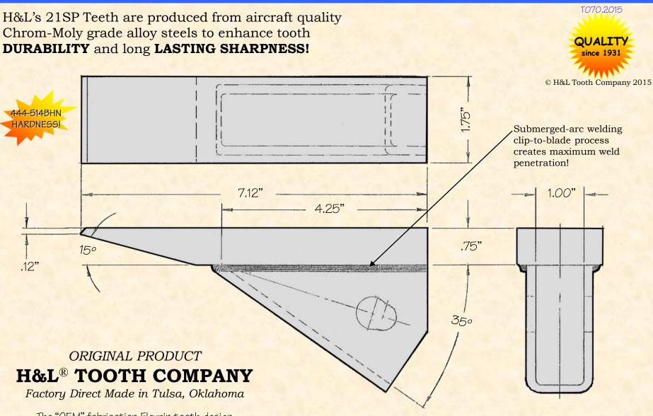
The "OEM" fabrication Flexpin tooth design
