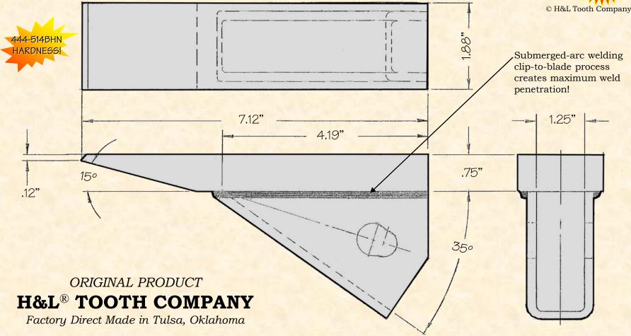
The "OEM" fabrication Flexpin tooth design
