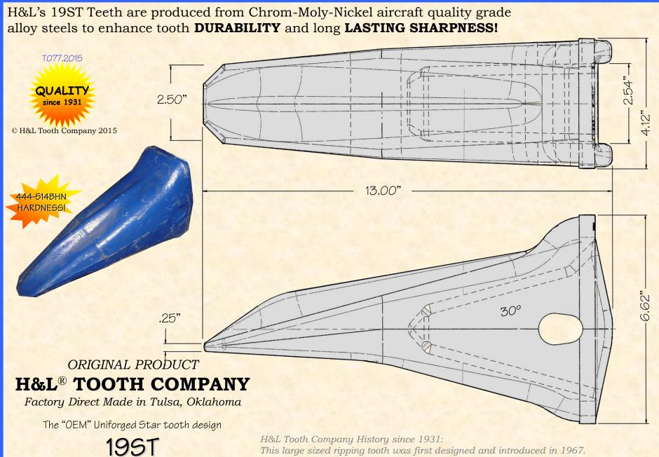
Ripping Star Tooth 27.5#/12.51kgs. This large sized ripping tooth was first designed and introduced in 1967. H&L's Star ripping Tooth was developed and forged at the Hi-Pro Forge Plant, a Division of the H&L Tooth Company in Montebello, California. The Tooth was originally designed to fit several Fiat-Allis Ripper Models of the day.
