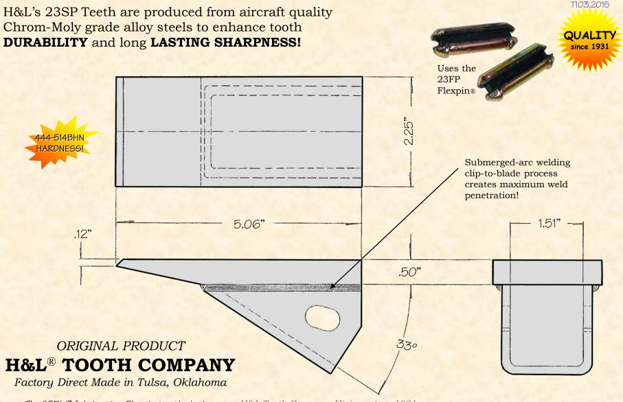
The "OEM" fabrication Flexpin tooth design
