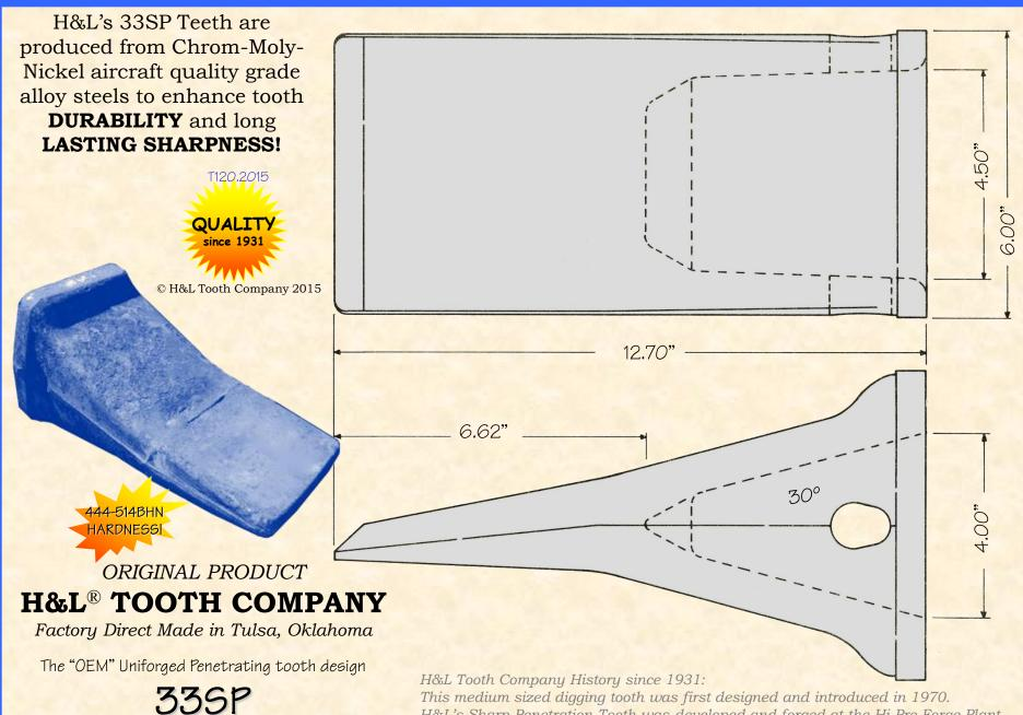
Sharp Penetration Tooth 43.4#/19.71kgs. This medium sized digging tooth was first designed and introduced in 1970. H&L's Sharp Penetration Tooth was developed and forged at the Hi-Pro Forge Plant, a Division of the H&L Tooth Company in Montebello, California. The Forged 33SP Tooth was originally designed for Wheel Loaders of the day like the Yale 8000.
