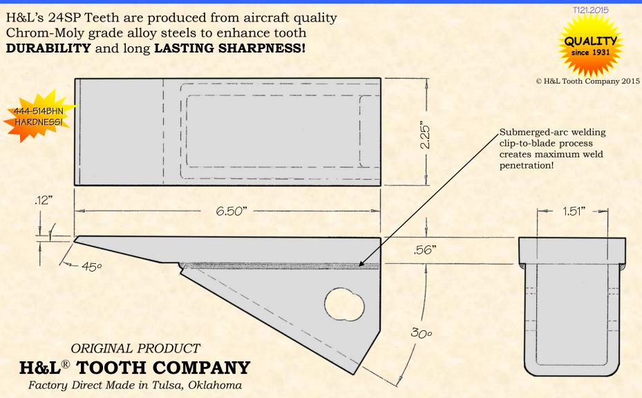
The "OEM" fabrication Flexpin tooth design
