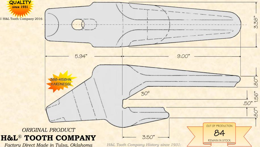
The "VP" Flexpin Style EXCAVATOR ADAPTER design
