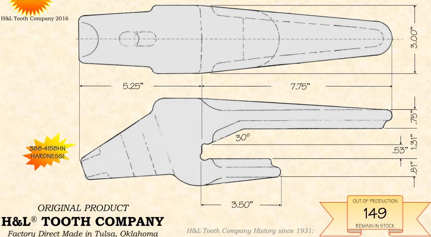
The "VP" Flexpin Style EXCAVATOR ADAPTER design
