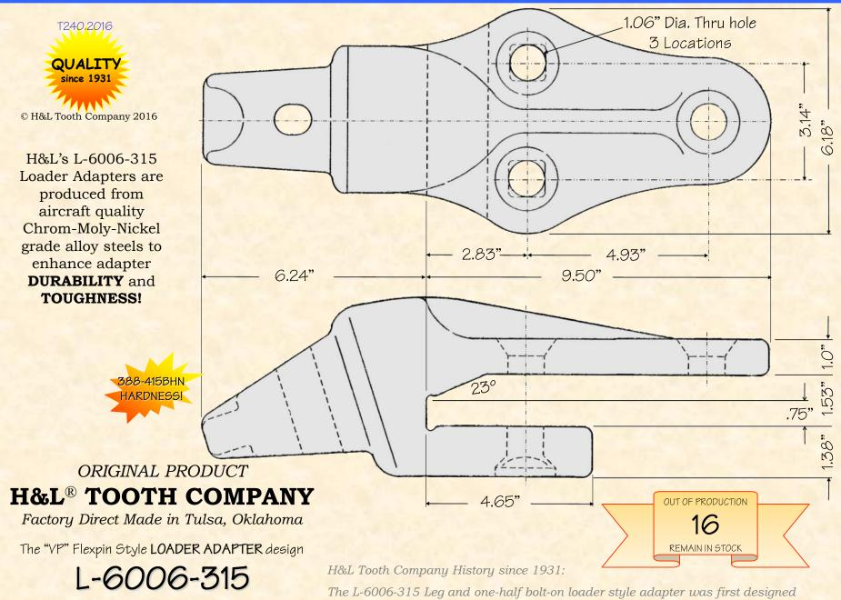
Loader Adapter 43.0#/19.5kgs. The L-6006-315 Leg and one-half bolt-on loader style adapter was first designed and introduced by H&L Tooth Company for Komatsu Models WA-350, WA-400 and WA-450 machines in 1986.
