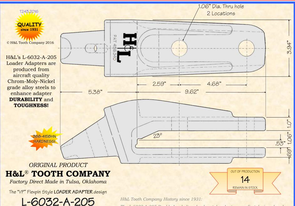
The L-6032-A-205 Double Leg bolt-on loader style adapter was first designed and introduced by H&L Tooth Company for Komatsu Models WA200 and WA-300 machines in 1988.
