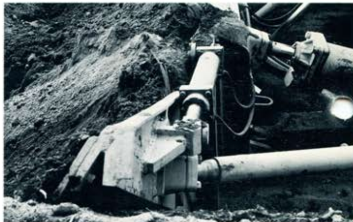
Side view showing lead of Sloper Blade, lead is adjustable forward to 1 1/2 ft. depending on type of material being cut.
