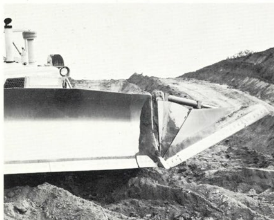
Photo shows SLOPER BLADE in lowest position (2:1) slope, revealing telescoping mole-board design arrangement which makes SLOPER BLADE "spill-proof." Clean slope toe allows precise sloping operation.
