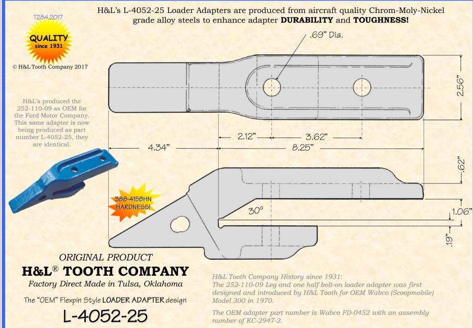
Loader Adapter 12.0#/5.44kgs. Today, H&L continues to produce the "Original" L-4052-25 adapter and 252-Series tooth system.
