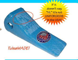
Tooth finishing starts with de-burring remaining flash materials prior to heat treating. Heat treatment consists of quench and temper for arend result of 514BHN in hardness.
