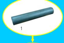
1. The "BILLET", a Chrom-Moly grade 17/16" raw steel diameter round, 7.50" long, is heated to 2250° F by electrical induction heaters.
