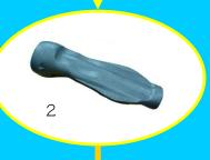
2. First pass in the 4" Upsetter balls the pocket area to ensure material flow into the tooth walls.
