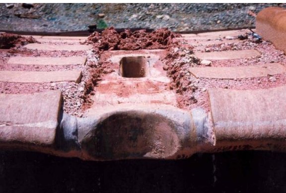
12 Months... The same stabilizer unit after 11.7 million tons of material has been removed.
