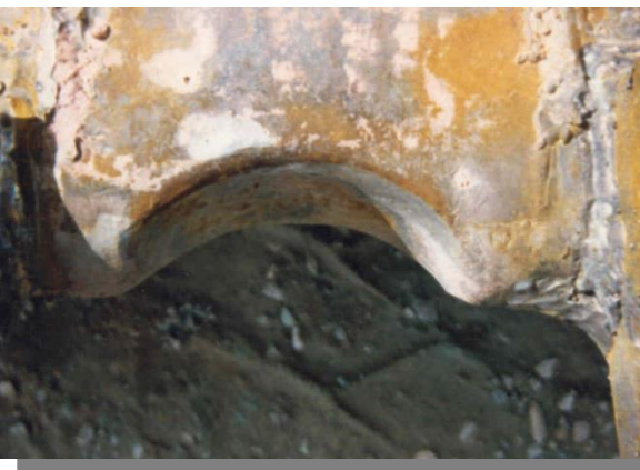
12 Months... The same stabilizer unit after 11.7 million tons of material has been removed.
