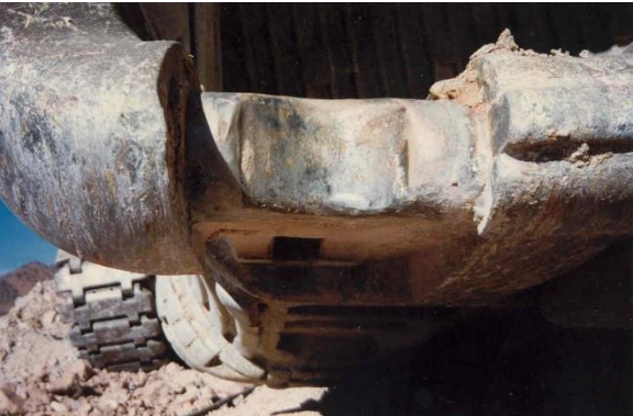
7 Months... The same stabilizer unit after 6.9 million tons of material has been removed.
