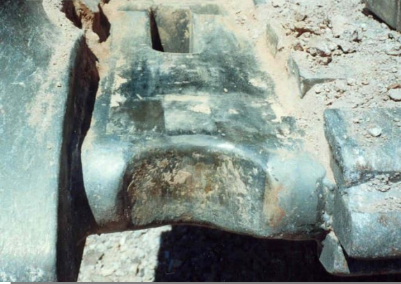
3 Months... CPS-10 stabilizer after 3.1 million tons of material moved.
