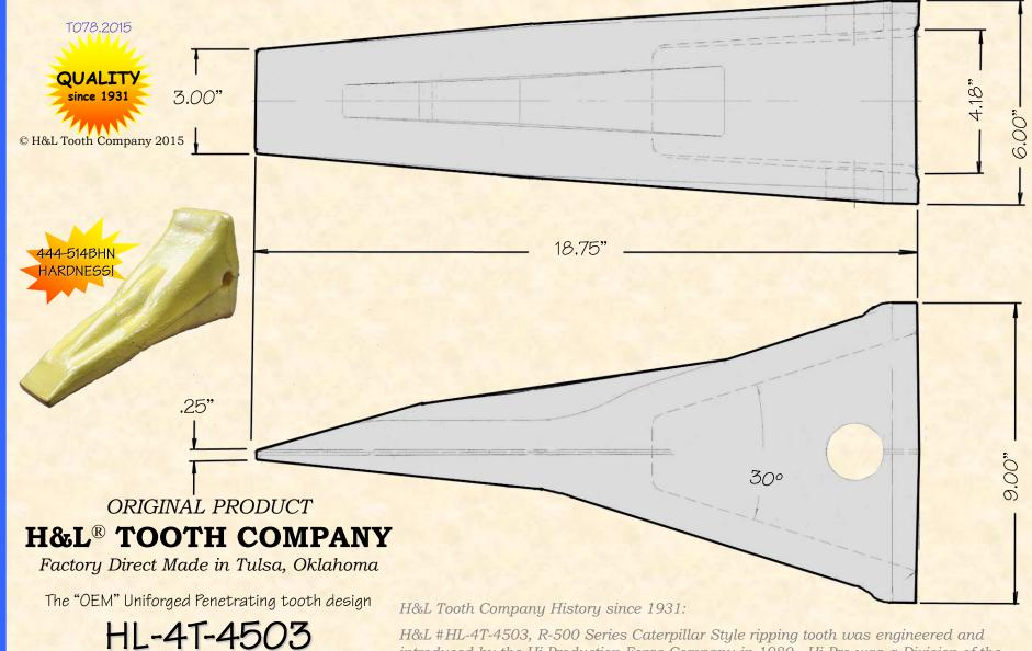
Ripping Penetration Tooth 66.0#/29.91kgs. H&L #HL-4T-4503, R-500 Series Caterpillar Style ripping tooth was engineered and introduced by the Hi-Production Forge Company in 1980. Hi-Pro was a Division of the H&L Tooth Company in Montebello, California during the 1970's and 80s. Replaces other numbers; 4T-4501, 4T-4502, 8E-8503, 4T-5501, 4T-5502.
