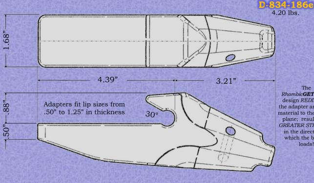
The Rhombic**GET**system design REDIRECTS the adapter and tooth material to the vertical plane; resulting in GREATER STRENGTH in the direction in which the bucket loads!
