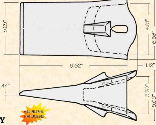
Uses the C-50 series Rubber Insert and Steel Pin
