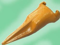
T - (Single Tiger) – The "T" is a V shape, ribbed non-centerline tooth for maximum penetration in applications such as frost or shale. It has improved wear life over other pick shaped designs and stays sharper longer for maximum value.
