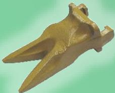
TVIP - The (Twin Tiger) is a double V shape, ribbed non-centerline tooth with excellent penetration. It is designed to be used in corner positions in conjunction with the Single Tiger design to cut clearance for bucket sides.
