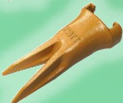
TT - The (Twin Tiger) is a double V shape tines with ribbed non-centerline tooth with excellent penetration. It is designed to be used in corner positions in conjunction with the Single Tiger design to cut clearance for bucket sides.
