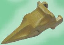
VIP or VIPL- (Single Tiger) – The “VIP” is a V shape, ribbed non-centerline tooth for maximum penetration in applications such as frost or shale. It has improved wear life over other pick shaped designs and stays sharper longer for maximum value.
