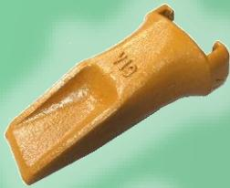
General purpose tooth no post identification is similar to the Long Paneled design. The Long Panel style tooth is for a medium abrasion applications with a deep designed recessed panel on the top surface for the tooth to stay sharp during the life of the GET.
