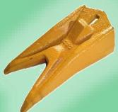
TVIP - The (Twin Tiger) is a double V shape, ribbed non-centerline tooth with excellent penetration. It is designed to be used in corner positions in conjunction with the Single Tiger design to cut clearance for bucket sides.
