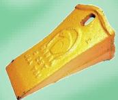
T – The “T” is a dual purposed tooth which change the digging pitch of the tooth by reversing. It is used for flush cut in normal position for general purpose applications or can be turned upside down for more aggressive digging.
